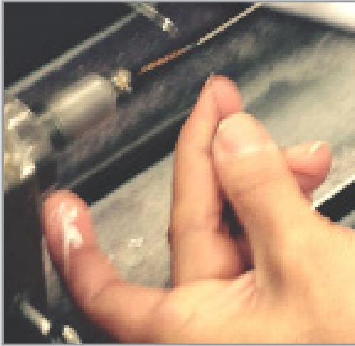
"Silking" the string with a delicate strand of colored thread to protect it from abrasion and help identify pitch. In a highly skilled step, the operator applies a small amount of glue (visible on her index finger at lower right) to hold the strand in place during winding.
